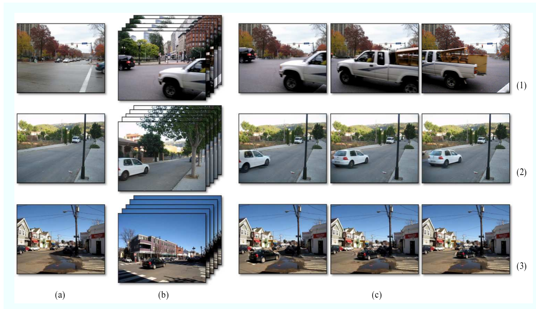
Figure 6. Category-level scene alignment applied to motion synthesis via object transfer. Query still image (a), the top video match of a scene containing moving objects (b), and representative frames from the synthesized sequence (c) obtained by transferring moving objects by computing dense correspondence from the video to the still query image.
