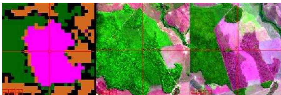
Figure 2. Left image: classification of low resolution data with the ENVIAIR software (forest in green, pasture in orange, deforestation in pink). Middle and right images: control using two high resolution Landsat images, acquired before and after the low resolution image. The deforestation is clearly visible from the center to the right images.
