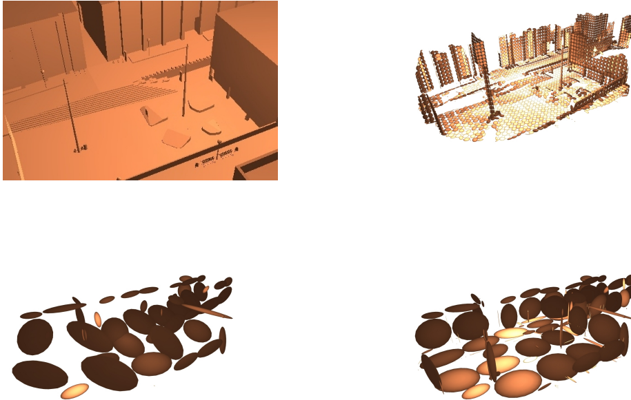
Figure 9. Top left: original scene. Top right: fine scale of the map. Bottom left: coarse scale of the map, one Gaussian per cell. Bottom right: coarse scale of the refined map with our clustering approach
