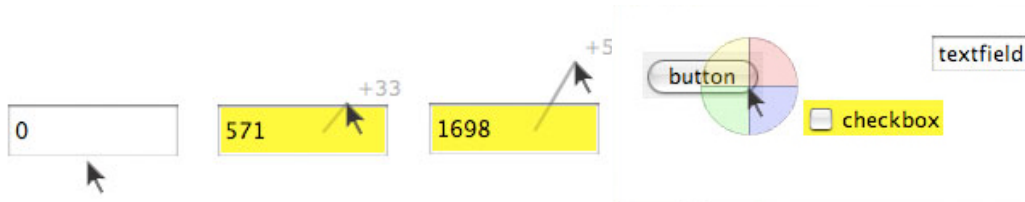
Figure 5. A numeric text field whose value can be set by a joystick-like interaction (left) and a semi-transparent menu to change the background color of Swing widgets (right)
