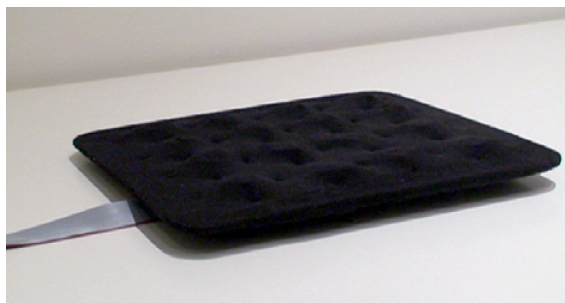
Figure 15. BubbleWrap simulates hardness by expanding and contracting fabric cells using electromagnetic force
