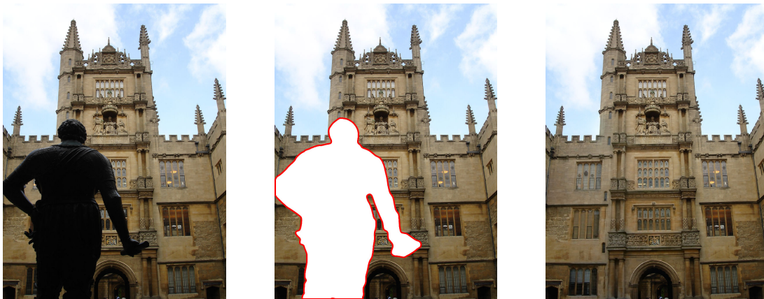
Figure 4. Automatic inpainting using photographs of the same scene downloaded from the Internet. From left to right: Original query image, target region to replace, result from the system. The replaced region is consistent with the rest of the original image and the boundary between is effectively hidden, producing a convincing result. Note the complexity of image structures on the inpainted facade.
