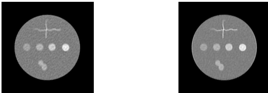
Figure 20. Results of Richardson-Lucy deconvolution using one image (on the left) and two images (on the right).
