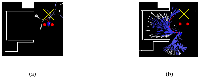
Figure 11. Change in the behavior of the autonomous wheelchair. In (a) the navigation don't take in account the personal spaces nor the Vis-a-vis formation, (b) the wheelchair have more information and respect the social conventions of space.
