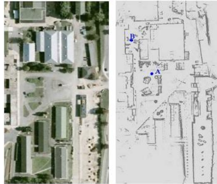
Figure 3. Bird view of INRIA Rocquencourt and the corresponding SLAM-based built global map
