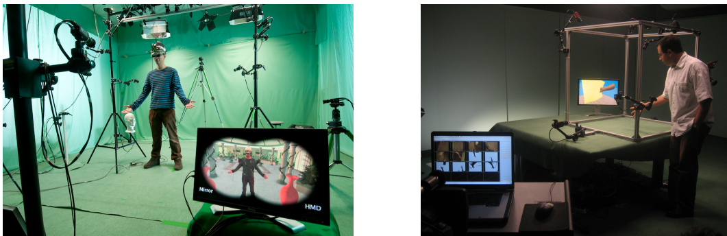
Figure 1. Left: The Grimage platform allows immersive/interactive applications such as this one. The real character is reconstructed in real-time and immersed in a virtual world, such that he/she can interact with virtual objects. Right: The mini-Grimage platform holds on a table top. It uses six cameras connected to six mini-PCs and to a laptop.
