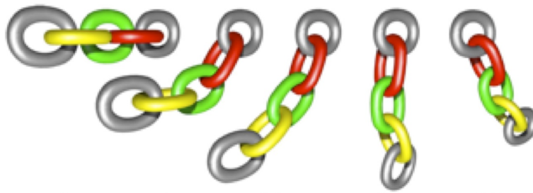
Figure 4. Animation of a chain combining a FEM model, a mass-spring model, a FFD grid, and a rigid body. This example is a perfect illustration of the flexibility of SOFA. Not only several algorithms for rigid or deformable bodies can be part of the same simulation, but they can also interact in a physically correct manner. No constraints between links were pre-defined, instead we relied on collision detection and stiff contact forces to handle the contacts. Using implicit integrator handling dynamically-created groups of interacting objects resulted in a stable simulation
