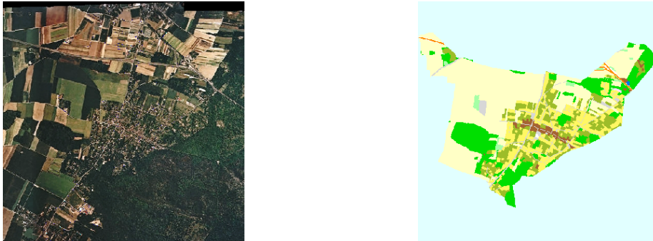
Figure 5. Image registration for the evaluation of retrieval systems. Left: mosaicked aerial image data; right: registered ground truth classification.
