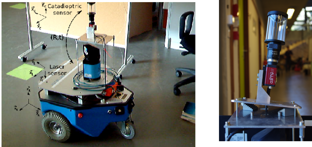
Figure 2. Left: Robot used for the experiment – Right: The omnidirectional camera mounted with a rotational offset
