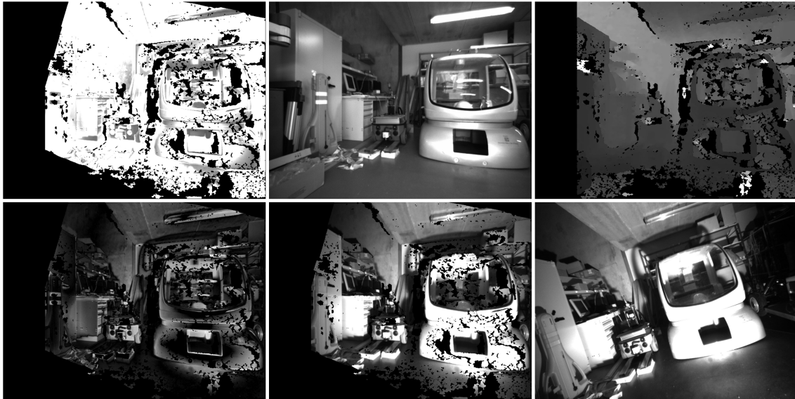
Figure 5. Top left, robust outliers weights. Top center, augmented reference image. Top right, reference depth-map. Bottom left, intensity error after alignment. Bottom center, registered image. Bottom right, original current image.
