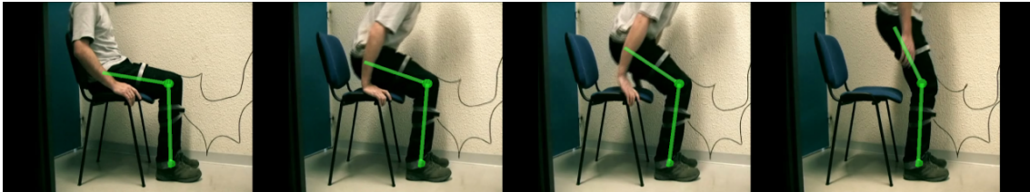
Figure 5. Angles estimated using inertial sensors in a sit-to-stand task.
