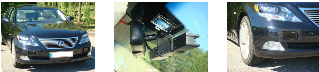
Figure 7. Lexus LS600h car equipped with two IBEO Lux lidars, a TYZX stereo camera, and an Xsens MTi-G inertial sensor with GPS.
