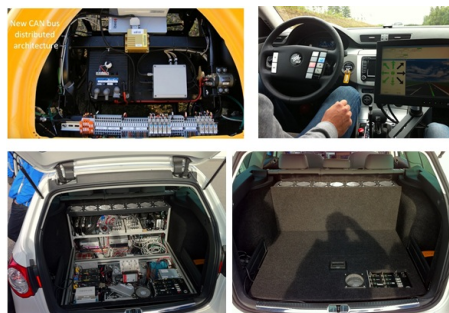
Figure 1. The Co-Pilot system in the Joint system architecture and HAVEit's FASCar demonstrator
