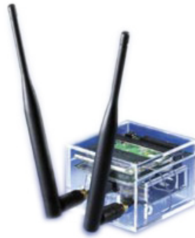
Figure 2. The device used for V2V and V2I wireless communications.
