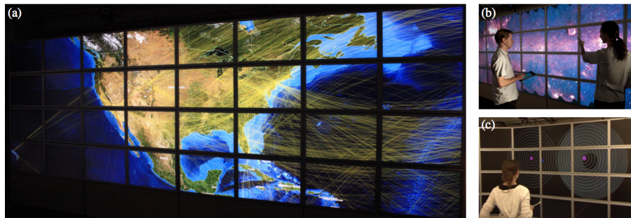
Figure 1. jBricks applications running on the WILD platform (32 tiles for a total resolution of 20\,480 \times 6\,400 pixels). (a) Zoomed-in visualization of the North-American part of the world-wide air traffic network (1 200 airports, 5 700 connections) overlaid on NASA's Blue Marble Next Generation images ( 86\,400 \times 43\,200 pixels) augmented with country borders ESRI shapefiles. (b) Panning and zooming in Spitzer's Infrared Milky Way ( 396\,032 \times 12\,000 pixels). (c) Controlled laboratory experiment for the evaluation of mid-air multi-scale navigation techniques.
