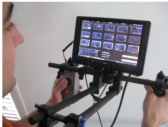
Figure 6. Director's Lens: a new workflow for interactive virtual cinematography. For a spatial partition analysis of a 3D environment, our tools automatically generates ranges of viewpoint suggestions following classical cinematographic conventions. Cameramen then select the suggestions and refine them using a 6DOF tracked device.
