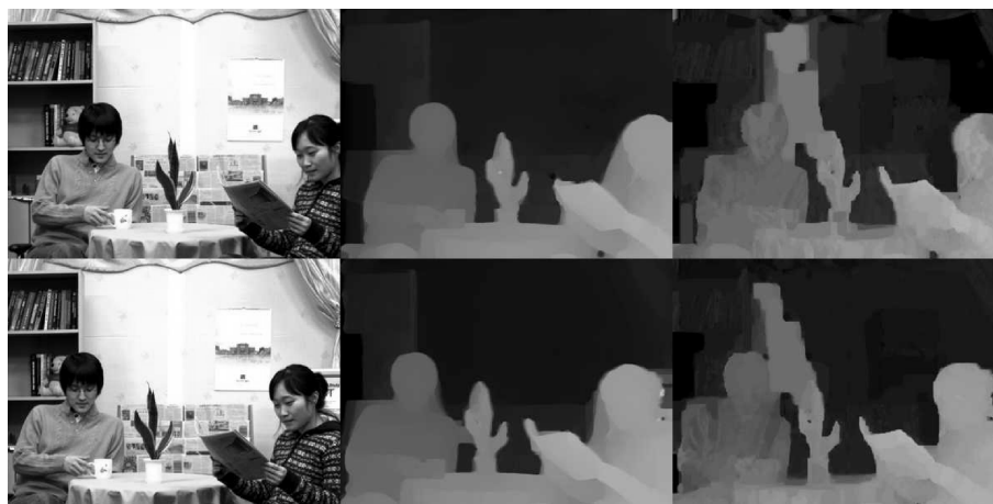
Figure 1. Depth maps extracted for the kendo sequence (right and left views) with DERS (3rd column) and TEMICS software (middle column).
