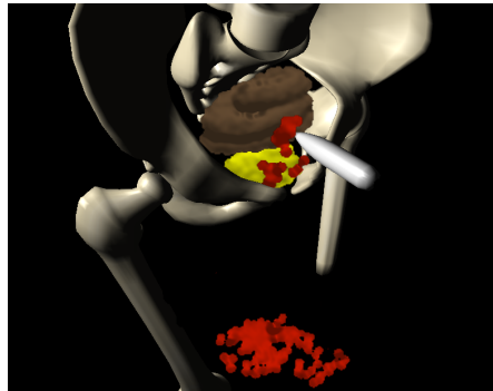
Figure 9. 6DoF haptic interaction in a medical scenario. Fluid blood pours from the deformable intestine when the user penetrates it with the rigid probe.
