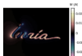
Figure 8. The field measured in Figure 6 is inverted, assuming that the sample is unidimensionally magnetized along the direction D_2 . The letters "ria" are fairly well recovered while the rest of the letters is blurred (because the hypothesis about the direction of magnetization is false for "In").
