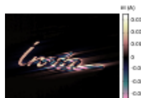
Figure 7. The field measured in Figure 6 is inverted, assuming that the sample is unidimensionally magnetized along the direction D_1 . The letters "In" are fairly well recovered while the rest of the letters is blurred (because the hypothesis about the direction of magnetization is false for "ria").
