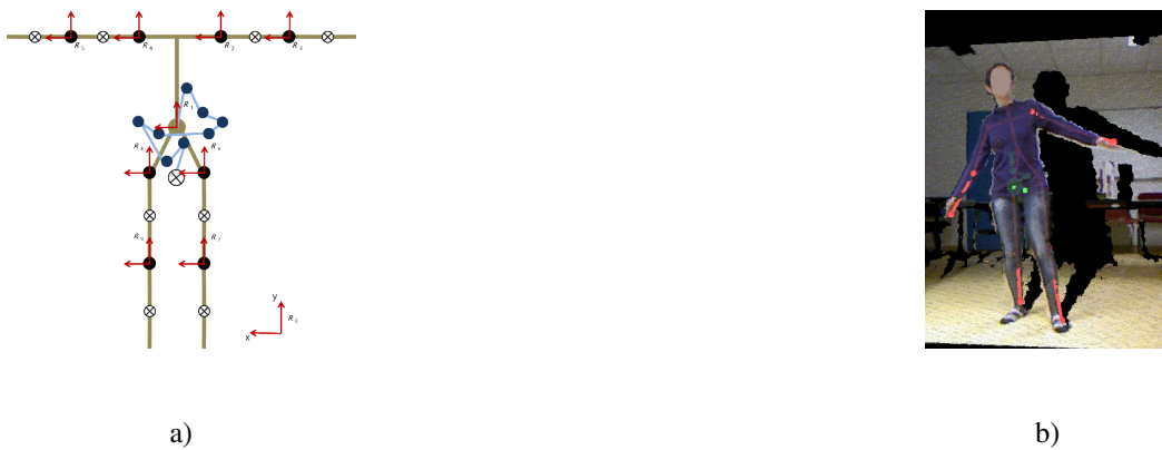
Figure 1. Center of mass estimation can be done using the statically equivalent serial chain. We assume a 9 rigid-link model (a) with spherical joints, capable of three dimensional movements. The SESC estimation can be performed in real time and is driven by joint angular measurements (b).
