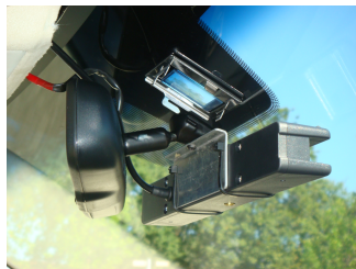
Figure 12. Lexus LS600h car equipped with two IBEO Lux lidars, a TYZX stereo camera, and a n Xsens MTi-G inertial sensor with GPS.
