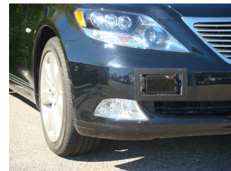
Figure 12. Lexus LS600h car equipped with two IBEO Lux lidars, a TYZX stereo camera, and a n Xsens MTi-G inertial sensor with GPS.
