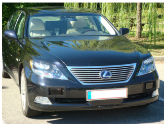
Figure 12. Lexus LS600h car equipped with two IBEO Lux lidars, a TYZX stereo camera, and a n Xsens MTi-G inertial sensor with GPS.
