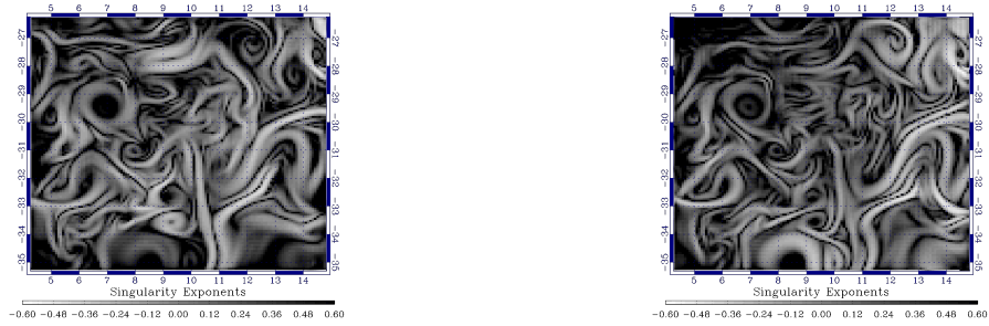
Figure 4. Local Predictability Exponents (LPEs) of ROMS-simulated p_{CO_2}^{ocean} signal (left) and of corresponding SST (Sea Surface Temperature) generated signal (right). Transitions are visually and quantitatively correlated, although not the same.
