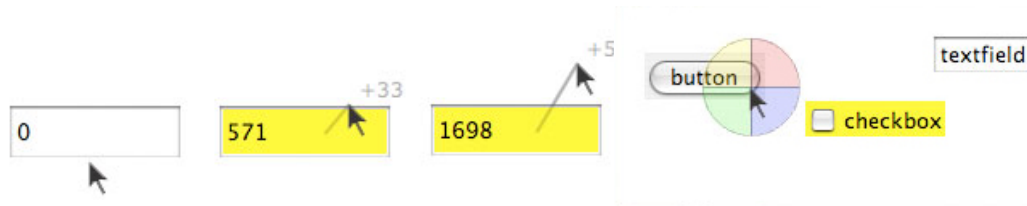
Figure 3. A numeric text field whose value can be set by a joystick-like interaction (left) and a semi-transparent menu to change the background color of Swing widgets (right)
