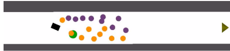
Figure 12. Navigation among crowds. The robot (rectangle) needs to reach the right side of the corridor. 2 groups of people (one in yellow, the other in blue) are crossing in this corridor. A classical motion planning would not find a path. The robot choses a leader (represented by a green circle around a person) and follows him.
