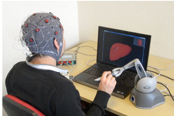
Figure 9. Medical simulator adapted to a BCI output. The user manipulates a virtual needle and has to insert it into a virtual liver to reach a tumor. Visual and haptic assistances are activated when a high mental workload is detected which corresponds to a more difficult manipulation of the needle.
