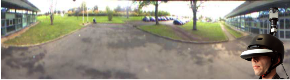
Figure 2. The “FlyVIZ” enables humans to experience in real-time a 360-degree vision of their surroundings.
