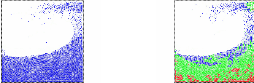
Figure 7. A dam break simulation with 5000 particles simulated with WCSPH (on the left) and with our adaptive method (on the right). On the right image, blue corresponds to full-dynamics particles, green to transition particles and red to restrained particles.
