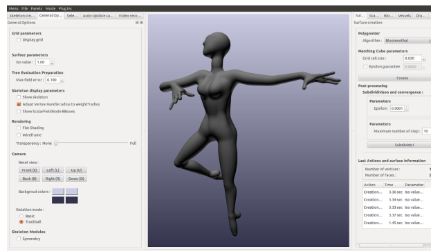
Figure 3. GUI and Example of implicit surface and modeled with the Expressive platform.
