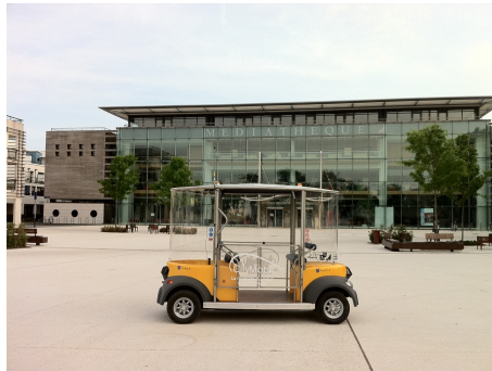
Figure 3. The Cybus operated at La Rochelle City during 3 months as a free transport service.
