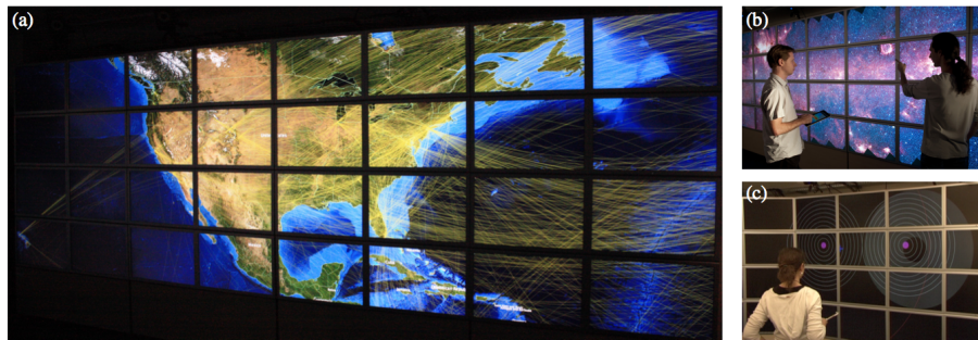
Figure 2. jBricks applications running on the WILD platform (32 tiles for a total resolution of 20\,480 \times 6\,400 pixels). (a) Zoomed-in visualization of the North-American part of the world-wide air traffic network (1 200 airports, 5 700 connections) overlaid on NASA's Blue Marble Next Generation images ( 86\,400 \times 43\,200 pixels) augmented with country borders ESRI shapefiles. (b) Panning and zooming in Spitzer's Infrared Milky Way ( 396\,032 \times 12\,000 pixels). (c) Controlled laboratory experiment for the evaluation of mid-air multi-scale navigation techniques.
