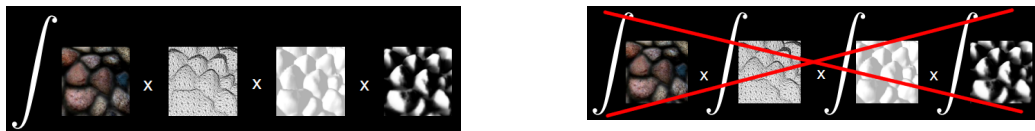
Figure 11. The resulting pixel color is the integral of the local rendering on the surface, which combines 4 fields which are: the color texture parameter, the visibility from eye, the visibility from light, and the shading. As these are varying and non-linear, the ubiquitous simplification of averaging each term separately is not valid.
