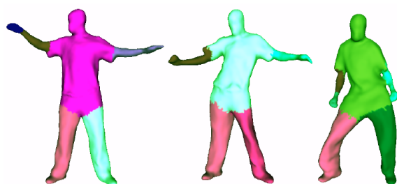
Figure 9. Segmentation of temporal mesh sequences into rigidly moving components.
