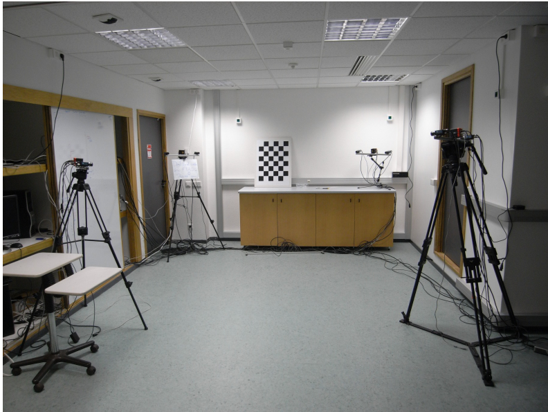
Figure 1. The mixed multi-camera system composed of four TOF-stereo sensor units.
