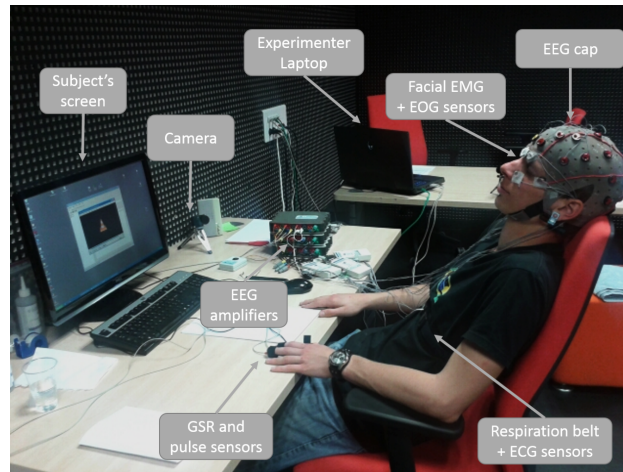
Figure 9. The setup of the experiment to induce and measure mental and psychosocial stress.
