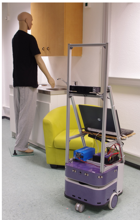
Figure 7. Robotic platform within the home-like environment for mobile RGBD experiments.
