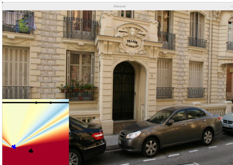
Figure 5. This interactive navigation tool shows an inset (in the lower left) that predicts comfort ratings for all possible camera orientations as seen from the blue camera's viewpoint. The application also restricts the user's motion to regions with acceptable predicted quality (in blue and yellow).
