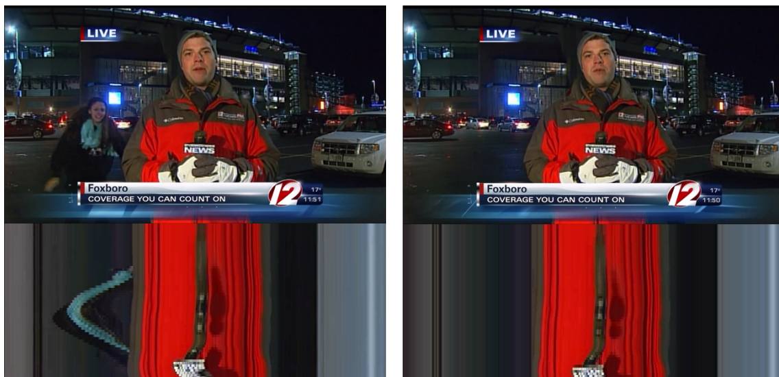
Figure 14. Inpainting task. Left : Original video (top) and xt slice (bottom) showing trajectories. Right : Our result. Clusters of fibers were computed and selected with only 7 mouse clicks to distinguish the disturbing girl from the reporter and background. The girl was removed and the hole was filled by extending the background fibers in time.
