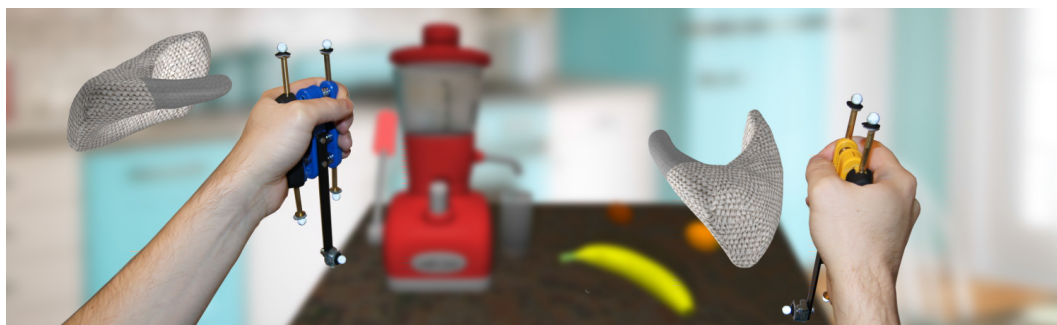
Figure 2. The Virtual Mitten : Visuo-haptic manipulation as enabled by our novel approach called the “Virtual Mitten”. Each hand holds an elastic device to control a virtual mitten (in grey) enabling the grasp of virtual objects.
