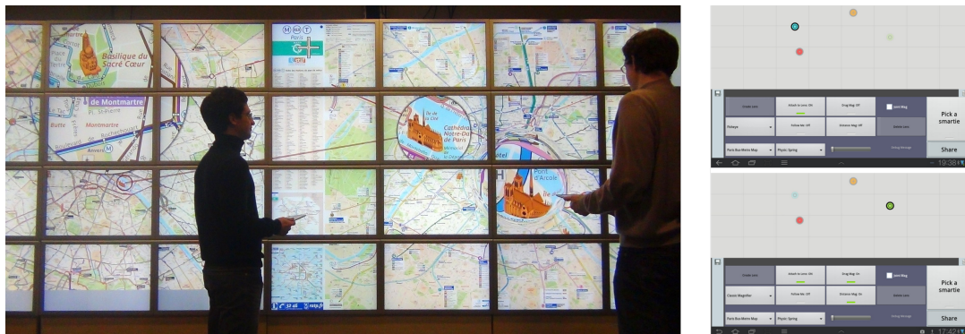
Figure 2. Left: Multiple Lenses, starting from the left a magnification lens, a DragMag and a fisheye. Right: two synchronized Smarties clients running on tablets. The four colored pucks are attached respectively to a magnification lens (left of wall), the anchor and lens of a DragMag (middle) and a fisheye (right). The active puck is the blue for the device on top, and green for the bottom. The described widgets added by the application are seen on the widget area.
