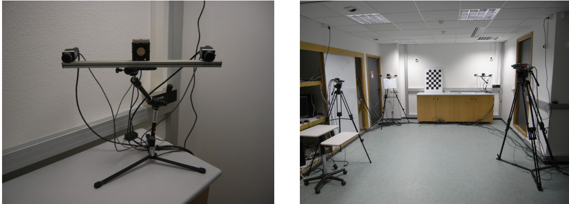
Figure 2. The MIXCAM laboratory is a multiple-camera multiple-PC hardware/software platform that combines high-resolution color (RGB) cameras with low-resolution time-of-flight (TOF) cameras. The cameras are arranged in “units”, where each unit is composed of two RGB cameras and one TOF camera (left image). Currently the system is composed of four such units (right image), or a total of eight RGB and four TOF cameras. Over years, in collaboration with 4D View Solutions, we have developed and maintained software packages for camera, multiple-camera, and cross-modal calibration, 3D reconstruction, multiple-camera stereo, TOF-stereo fusion, and image-based rendering.
