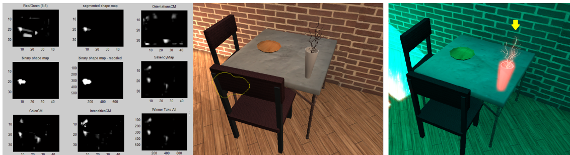
Figure 5. A low level saliency algorithm indicates that the most salient area of the image is the dark area behind the chair. Our tool highlights the vase at a consistent/singleton location as the most salient object in the image.
