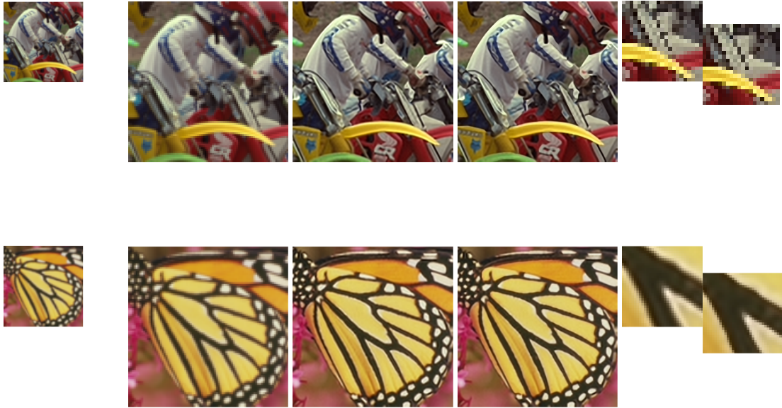
Figure 3. Comparison of SR results ( \times 3 ). (a) LR image; (b) Nearest-neighbor; (c) Sparse method without structure-based regularization; (d) SE-ASDS results. (e) Comparison between (c) and (d) on patches: edges of (d) are more contrasted than (c).
