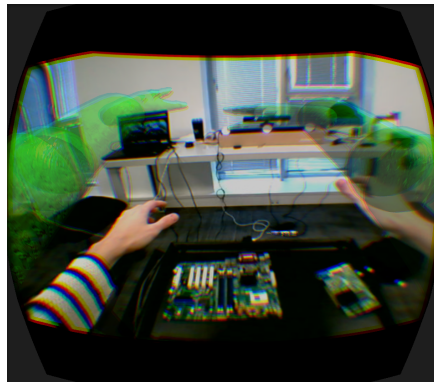
Figure 9. Remote collaborative maintenance using mixed reality.
