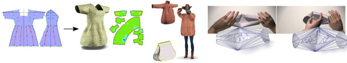
Figure 5. Example of developable model generation from sketches in [10] and for virtual paper interaction [14].
