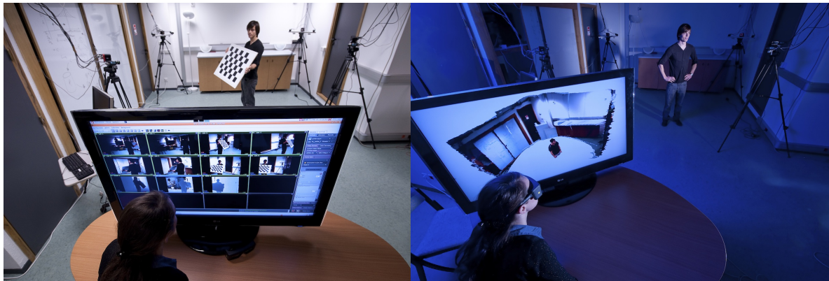
Figure 4. MIXCAM is a multiple-camera multiple-PC hardware/software platform that combines high-resolution color (RGB) cameras with low-resolution time-of-flight (TOF) cameras. The cameras are arranged in TOF-stereo “units”, where each unit is composed of two RGB cameras and one TOF camera. Currently the system is composed of four such units, or a total of eight RGB and four TOF cameras. In 2015 we completed algorithms and software packages for the calibration of individual TOF cameras [3] and of the whole system composed of four units, e.g. left image, [24]. The system allows high-resolution reconstruction of people, e.g. right image, [23].
