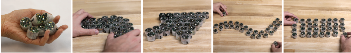
Figure 3. Zooids can be held as tokens, manipulated collectively or individually, behave as physical pixels, act as handles and controllers, and can move dynamically under machine control. They are building blocks for a new class of user interface we call swarm user interfaces.
