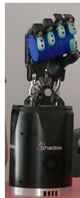
Figure 22. Closure posture of the Shadow robotic hand in the palmar grasp situation.
