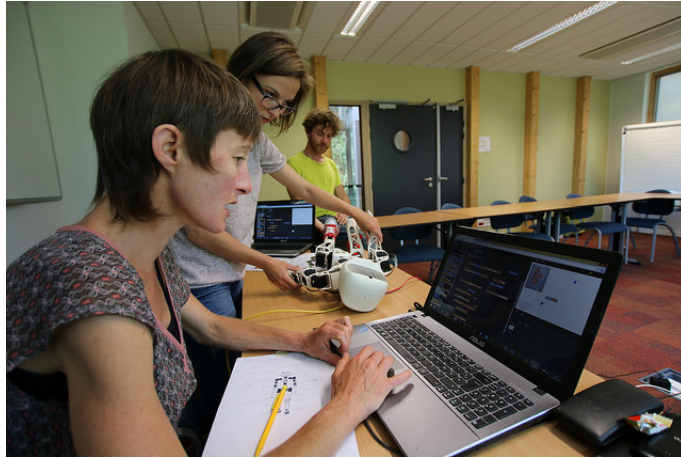
Figure 4. Using Snap! to program a robot by demonstration and create complex choreographies
