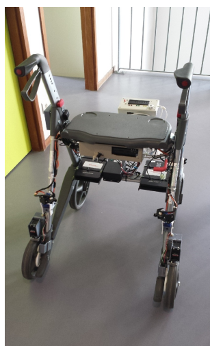
Figure 4. Rear view of the ANG-med walker with the 4 distance sensors that are used to monitor and assess rehabilitation exercises
