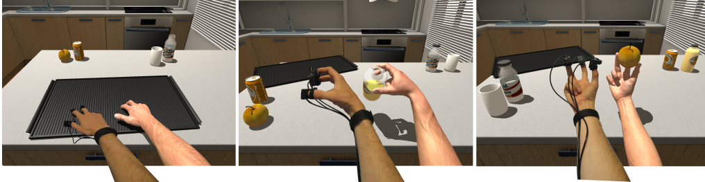
Figure 10. Illustrative use cases of our approach HapTip: the user can get in contact and tap a virtual bottle, touch a surface and feel its texture, and heft an object and feel its weight.
