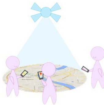
Figure 9. Sketch showing the Navidrone concept: users interact with maps projected from drones by using their phones.
